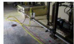
Installed ultrasonic transducer and clamp
